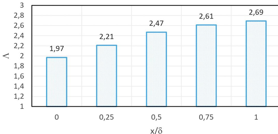
Fig. 5. Dependence of the of shear strain on the relative coordinate  $x/\delta$
