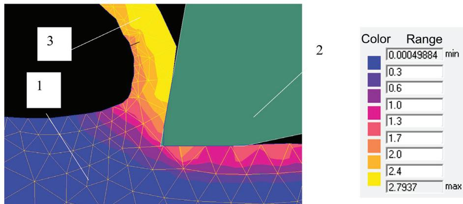
Fig. 3. Solution of the problem of separation of chips at an angle of  $\gamma = 10^\circ$  and a nominal removal depth of 1 mm:
