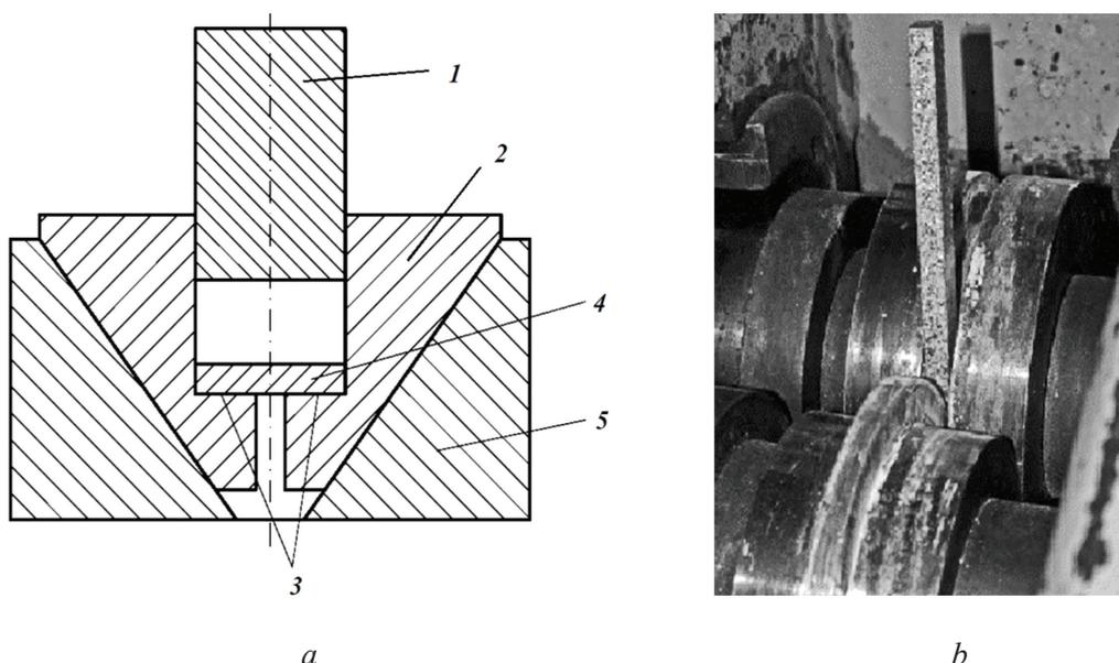
Fig. 1. Scheme of cold pressing of a billet made of chips (*a*) and a photo of subsequent hot processing on a combined rolling-pressing process unit (*b*)
