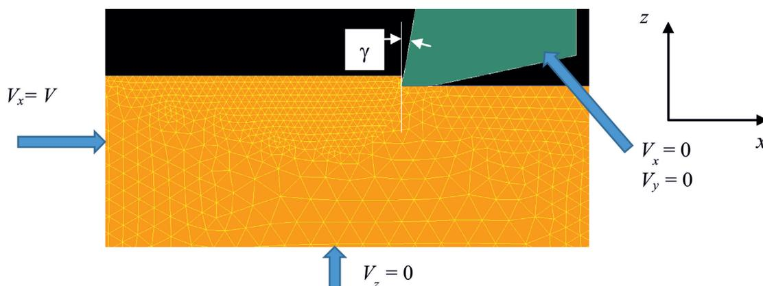
Fig. 2. Boundary conditions in the formulation of the problem and the coordinate system,  $\gamma$  – tool rake angle
