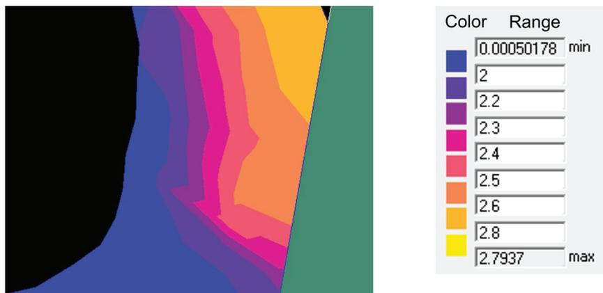
Fig. 4. Field of the of shear strain  $\Lambda$  in the place of separation of the chips from the cutter, on the right with a color key
