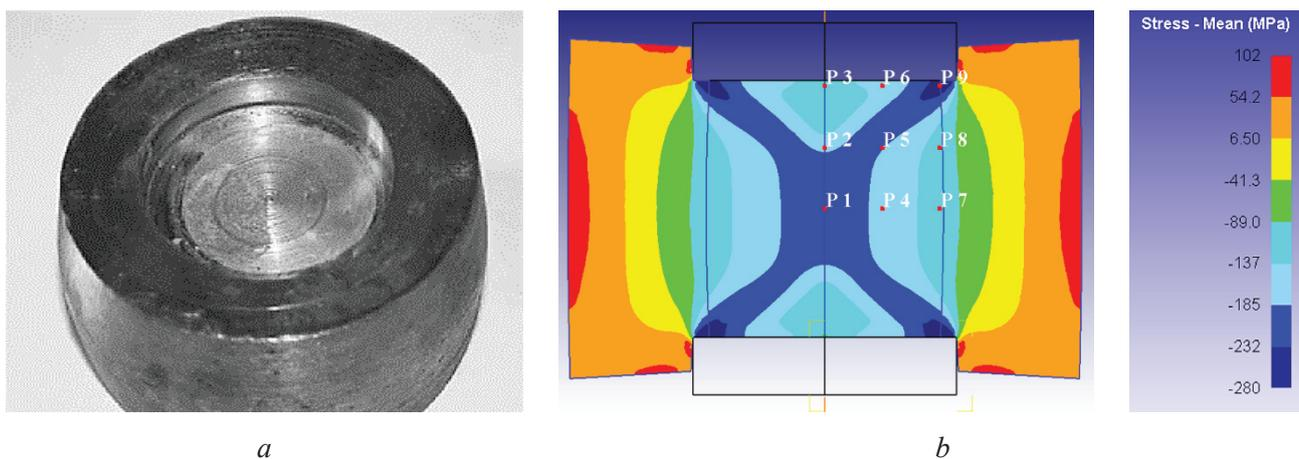
Fig. 1. Photo of the assembly (*a*) and calculation model of the process (*b*) upsetting of a magnesium billet in a shell with an estimation of mean stresses (stress mean)
