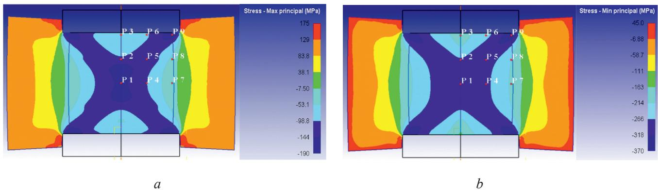
Fig. 3. Distribution of the maximum (a) and minimum (b) principal stress
