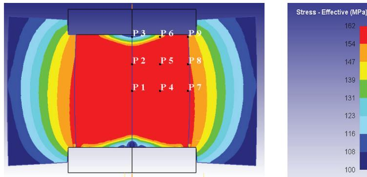
Fig. 2. The distribution of stress intensity
