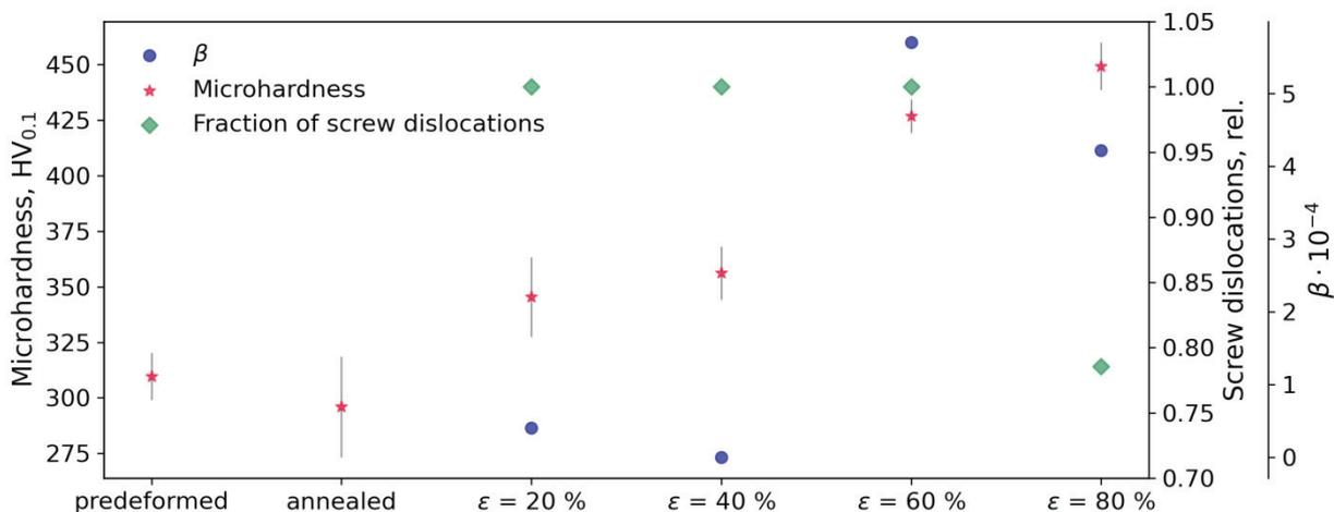
Fig. 6. Relative fraction of edge dislocations, parameter  $\beta$  and microhardness of the  $Al_{0.3}CoCrFeNi$  alloy during cold rolling
