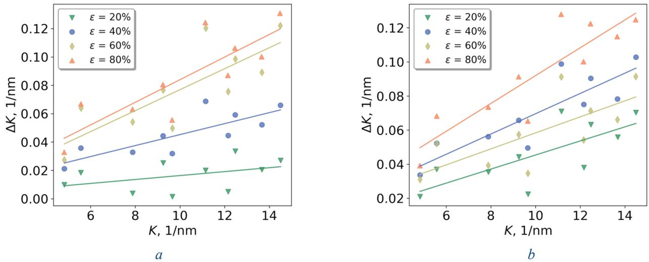
Fig. 2. Williamson-Hall plots for  $Al_{0.3}CoCrFeNi$  alloy after cold rolling for (a) RD and (b) TD directions
