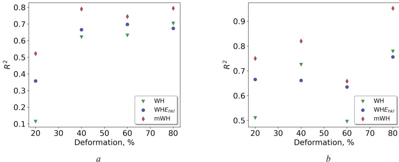
Fig. 5. The coefficient of determination for various peak profile analysis methods used in this study: the classical *Williamson-Hall* (WH) method; classical method corrected for the modulus of elasticity ( $WHE_{hkl}$ ); modified *Williamson-Hall* (mWH) method. The results for RD (a) and TD (b) directions are presented
