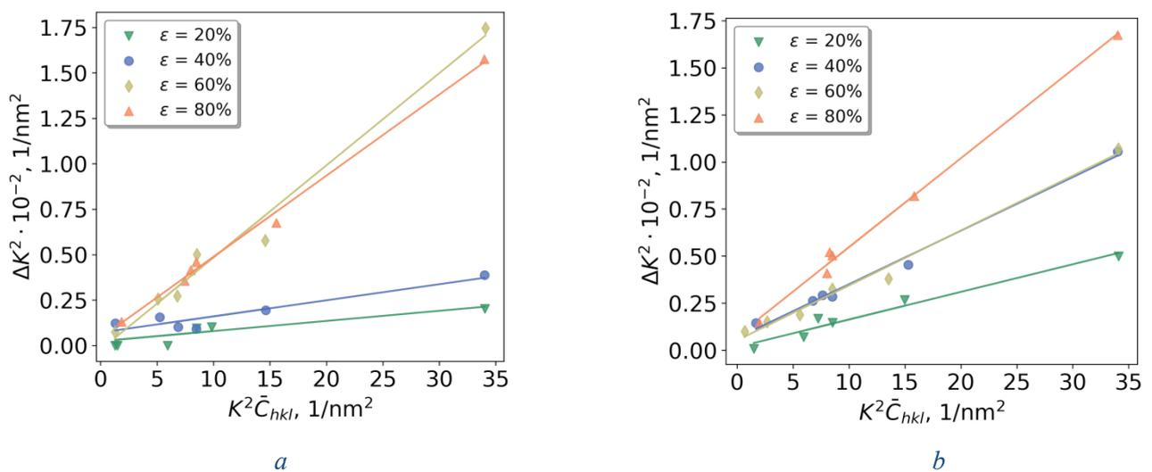
Fig. 4. Modified Williamson-Hall plots for  $Al_{0.3}CoCrFeNi$  alloy after cold rolling for (a) RD and (b) TD directions
