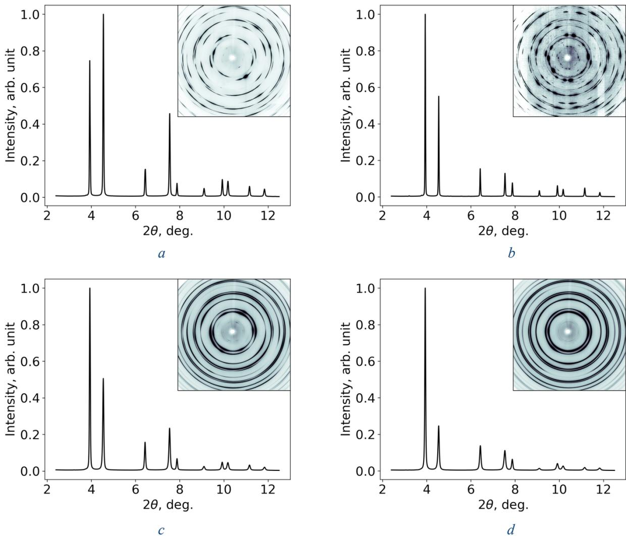
Fig. 1. X-ray diffraction patterns of the  $Al_{0.3}CoCrFeNi$  high-entropy alloy in pre-deformed state (a); after annealing at 400 °C (b); after cold rolling with 40 % (c) and 80 % (d) reduction
