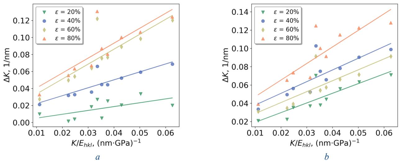
Fig. 3. Williamson-Hall corrected by elastic modulus plots for  $Al_{0.3}CoCrFeNi$  alloy after cold rolling for (a) RD and (b) TD directions
