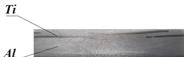
Fig. 3. Macrostructure of reinforced composite material based on light metals and alloys
