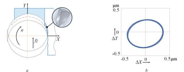
*Fig. 3.* Pattern of the passage of the cutting edges through the processing zone: a – the trajectory of the  $i^{th}$  tooth corresponding to the effective diameter of the tool; b – deviation trajectory of the front spindle support (*Formulated by the authors*)
