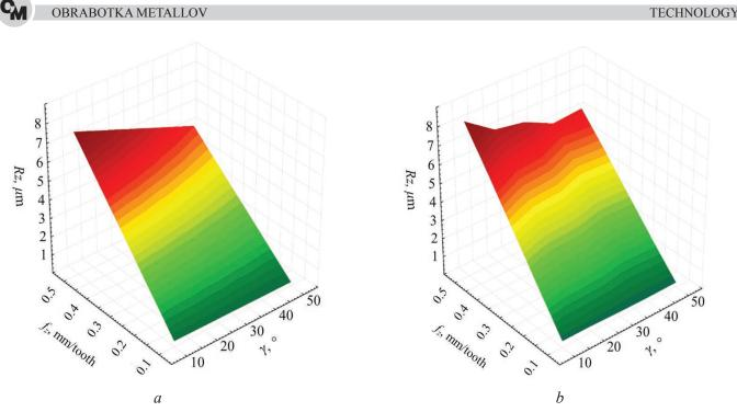
*Fig. 9.* Dependences of the roughness Rz on the feed and the angle of inclination of the tool: a – theoretical; b – experimental
