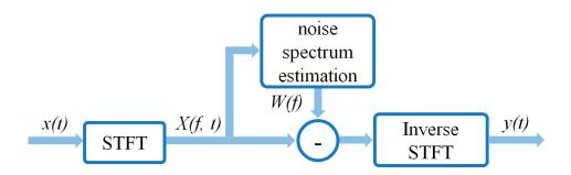
*Fig. 2.* The proposed spectral subtraction algorithm scheme: x(t) – original signal; *STFT* – Short Time Fourier Transform; W(f) – is the function of the weighting window; y(t) – transformed signal (*Formulated by the authors*)
