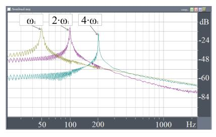
*Fig. 6.* Frequency response of harmonic sound waves obtained by milling with an inclination angle of 40° (*Formulated by the authors*)
