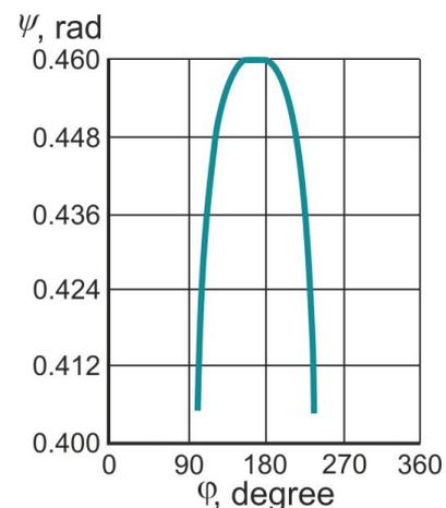
As can be seen from the above Option, the laws of change of kinematic parameters for the cam-rocker mechanism do not satisfy the set tasks of synthesis. Several other options were considered. The results of theoretical calculations are summarized in Table.
