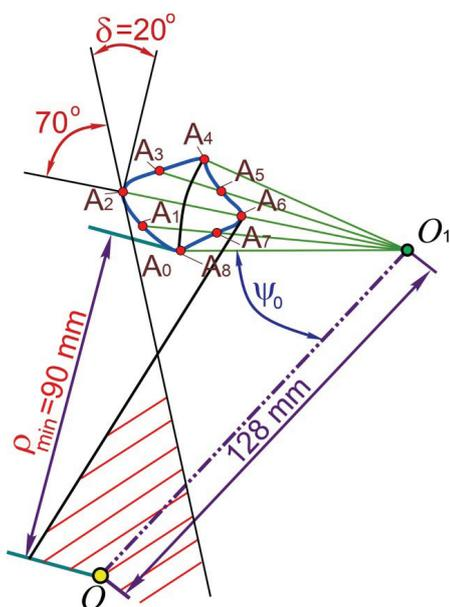
Fig. 4. To determine the missing parameters of the cam mechanism
