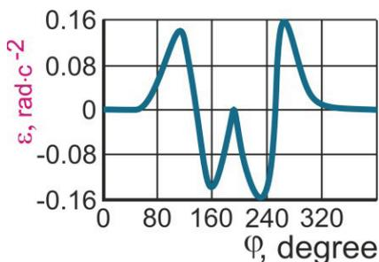
Fig. 11. Graph of the change in the accelerations of the rocker at  $\rho_{\min} = 70$  mm
