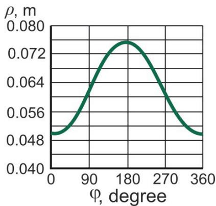
Fig. 12. Graph of the change in the numerical values of the radius vectors at  $\rho_{\min} = 50$  mm
