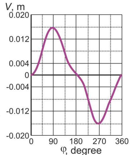
Fig. 3. Cam roller center velocity analogs
