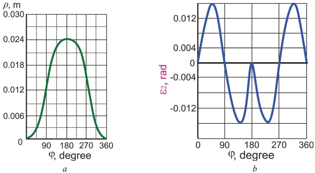
Fig. 5. Kinematic characteristics of the center of the roller for the cam mechanism:
