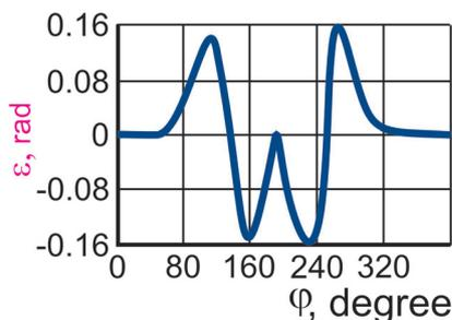
As can be seen from the graphs shown in Fig. 7 and 8, the swing and acceleration angles have smooth and continuous functions without oscillation. In Fig. 7, 8, there are dwells at the beginning and end of the graphs. Its total value is about  $80^\circ$ .
