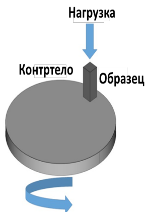
Fig. 2. Tribological loading scheme “pin-on-disc”
