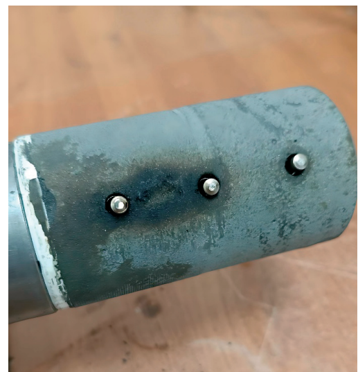
Fig. 2. Defect (failure) of the metal-polymer composite due to exceeding the permissible temperature limit for the metal-polymer
