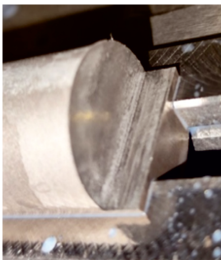
Fig. 5. Sample surface after machining with JJ Tools 4SUE080120S08
