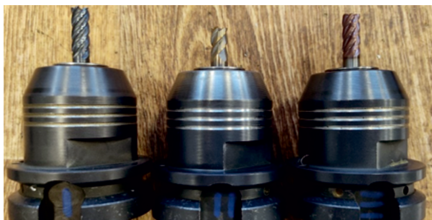
Fig. 3. Tool mounted in a SCHUNK hydroplastic holder
