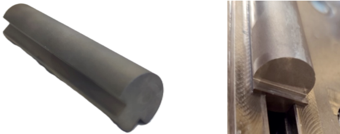
Fig. 2. Workpiece sample made of Mo-30TiC alloy with a technological shank
