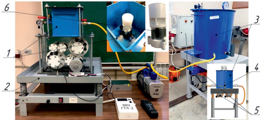
Fig. 2. Experimental setup for vibro-vacuum filling of internal cavities in SLM shells with a metal–polymer composite material ( MPCM ):
