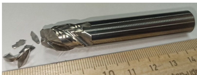
Fig. 11. Photograph of a typical fracture of the cutter teeth
