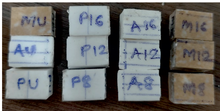
Fig. 1. Representative mechanical and tribological specimens of PTFE nanocomposites after cryogenic treatment
