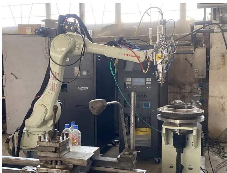
Fig. 2. Appearance of a robotic complex for laser cladding
