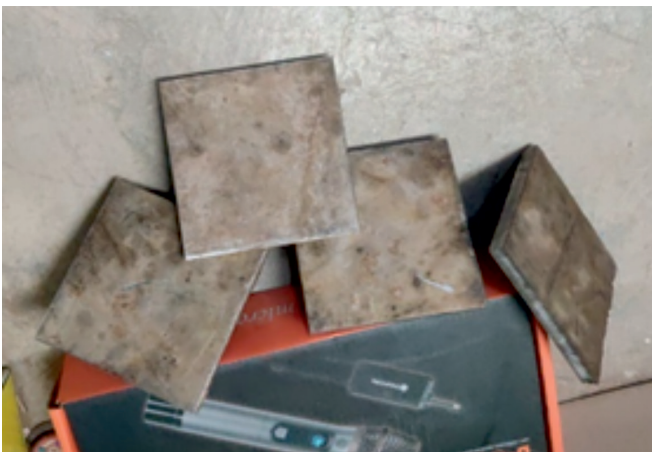
Fig. 1. Commercially pure titanium workpiece material used in the study
