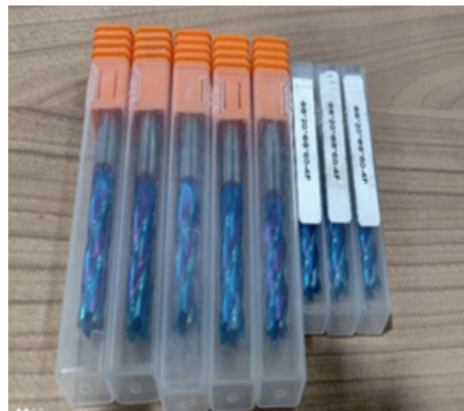
Fig. 2. WC-Co end mill cutters used in the investigation
