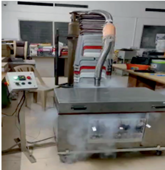
Deep cryogenic treatment conditions used for WC-Co cutting tools
