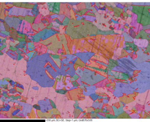
Fig. 3. Results of microstructural characterization of the surface layer of 1.1% C-13% Mn steel after shot peening:
