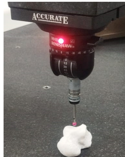
Fig. 7. Dimensions of the talus bone measured using a coordinate measuring machine (CMM)
